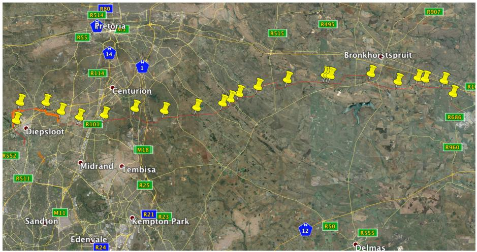
*Figure 18.* Route of proposed Bravo 3 power line, showing locations where bird flight diverters need to be fitted to the lines (see Table 5b)
